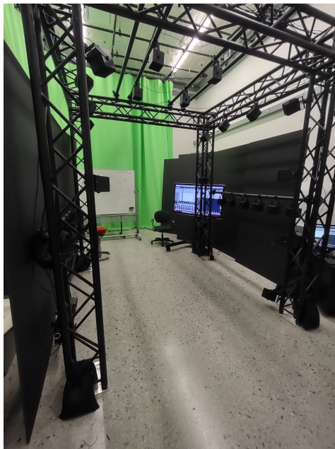
Figure 1: The Tesseract with 32 loudspeakers
